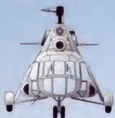
Mi-8 'HIP-A': The first Mi-8 was the single-engined prototype that lacked power and only had a four-bladed main rotor.
